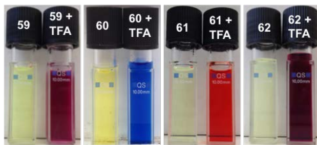
Figure 17. Color change of \text{CH}_2\text{Cl}_2 solutions of several quinazoline derivatives in the presence of TFA. Adapted with permission from reference [35] (copyright 2014 American Chemical Society).
