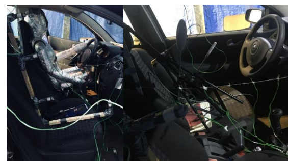
Fig. 4. Images during the experimental sessions with thermal manikin and CS
