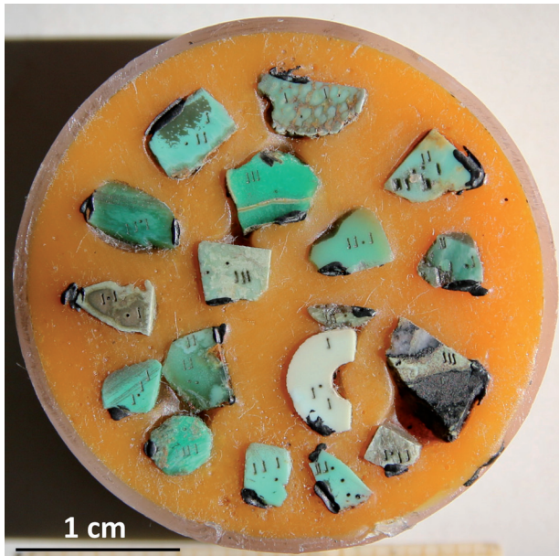
Fig. 4: Variscite archaeological samples after ICP-MS-LA analysis (SCID, Huelva University, 2002) A statistical approach was used looking for similarities between archaeological variscite samples and those coming from the above quoted Iberian geological localities.
