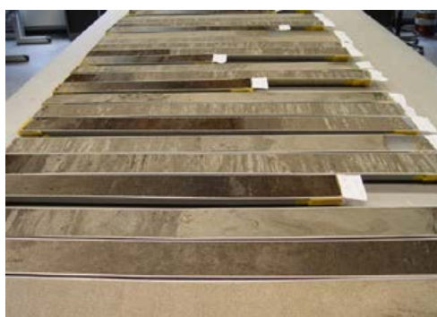
▲ Vibrocores undergoing analysis following extraction and splitting (courtesy Vos 2013, Deltares).
