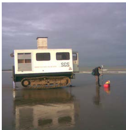
▲ Cone penetration testing on the beach at Raversijde (courtesy UGent).
