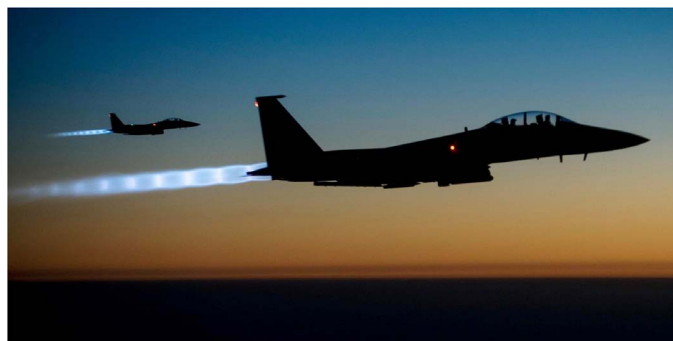
Fig. 3. Evidence for evenly spaced Mach disks in the supersonic exhausts of a pair of U.S. Air Force F-15E Strike Eagles flying over northern Iraq (credit: U.S. Air Force/Senior Airman Matthew Bruch).
