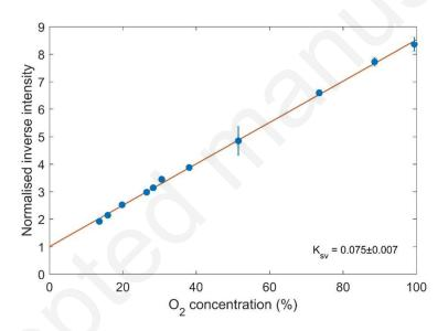
Fig. 5. Normalised inverse intensity signal  $I_0/I$  ( $I_0$  is the intensity signal in the absence of oxygen) as function of the oxygen concentration and linear fit to the Stern-Volmer equation, yielding a value of  $K_{SV} = 0.0752$  %<sup>-1</sup> of the Stern-Volmer constant.
