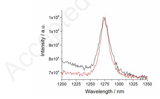
**Fig. 4.**  ${}^{1}\Delta_{g}$  O<sub>2</sub> emission spectra recorded upon irradiating of **1** with an excitation wavelength of 375 nm as a powdered sample (red) or in CH<sub>2</sub>Cl<sub>2</sub> solution (black).
