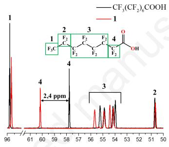
Fig. 1. <sup>19</sup>F NMR spectrum of  $CF_3(CF_2)_6COOH$  and 1.
