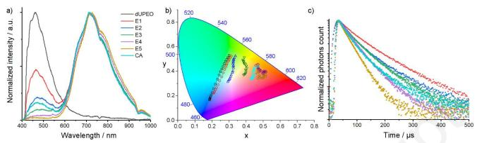
Figure 2.a) Normalized emission spectra of hybrid materials irradiated between 350-380 nm; b) CIE 1938 diagram coordinates for excitation ranging from 365 up to 450 nm; dUPEO (black), E1 (red), E2 (blue), E3 (green), E4 (purple, E5 (maroon) and CA (cyan); c) phosphorescence emission decay profiles recorded in the metal cluster emission range (662-798 nm).
