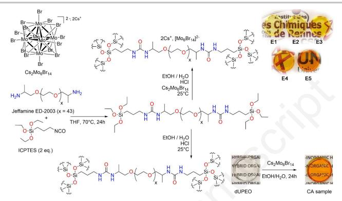
Figure 1. Structure of octahedral Cs<sub>2</sub>Mo<sub>6</sub>Br<sub>14</sub> metal cluster compound (1), diureasil PEO (dUPEO) hybrid sol and synthetic schemes for the preparation of unloaded and loaded dUPEO xerogel containing 1.
