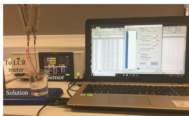
Figure 7. Experimental setup for testing of sulfate samples at different concentrations.
