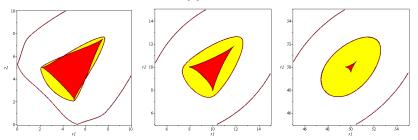
There are 4 solutions to the DKP in the yellow region (inside the small oval and outside the deltoid) and 8 in the red one (inside the deltoid). The deltoid is shrinking to a point as  $r_3$  tends to infinity, giving in the limit the picture of the degenerate DKP. There is also an oval of the curves of critical values which is not relevant for the analysis of the number of real solutions to the DKP; it disappears for the degenerate DKP.
