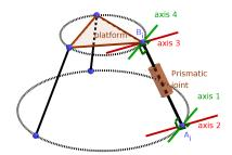
This small change changes drastically the kinematic behaviour of the platform. The configuration space now contains four modes of operation corresponding to 3-planes in the Study quadric, which are the modes  $\mathfrak{K}_1, \mathfrak{K}_2, \mathfrak{K}_3, \mathfrak{K}_4$  of the SNU, plus another "mysterious" mode which is a real subvariety of dimension 3 of the Study quadric whose computed ideal has a long list of generators:
