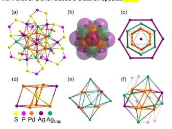
**Fig. 4** (a) Total structure of  $[Pd_6Ag_{14}S\{S_2P(O^nPr)_2\}_{12}]$  (2) with propoxy groups omitted for clarity. (b) The  $Pd_6Ag_{14}$  core. (c) View of the  $Pd_6Ag_{14}$  core along the  $C_3$  axis. (d) The sulfiderhombohedron. (f) The whole  $Pd_6Ag_{14}$  metal framework.
