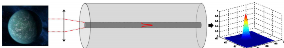
Fig. 19. Optical scheme of the detection of the MIR signal coming from an exo-planet through space. The beam profile on the right corresponds to a single-mode TAS glass at 10.6 \mu\text{m} . Reprinted with permission from Ref. [19].
