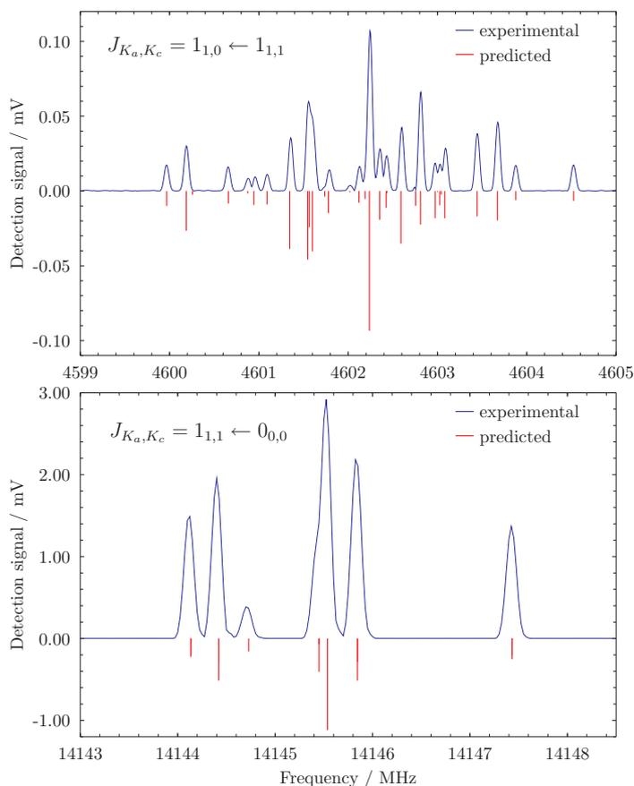
**Fig. 4.** Recordings (blue trace) of the  $1_{1,0} - 1_{1,1}$  (upper panel) and  $1_{1,1} - 0_{0,0}$  (lower panel) rotational transitions of imidazole taken with the COMPACT chirped-pulse spectrometer at DESY. The red histogram (inverted) indicates the predicted position of the hyperfine components computed using the spectroscopic parameters of Table 2.
