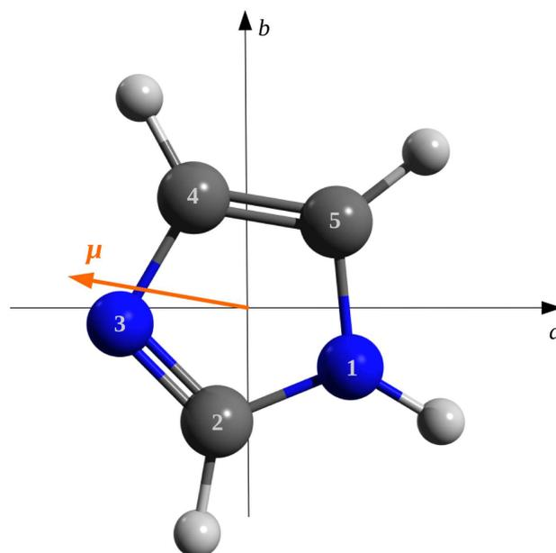
**Fig. 2.** Molecular structure and principal inertial axes of imidazole. The *c* axis is perpendicular to the *ab* molecular plane. The orange arrow indicates the direction of the electric dipole moment  $\mu$  and points towards the displacement of the notional negative charge.
