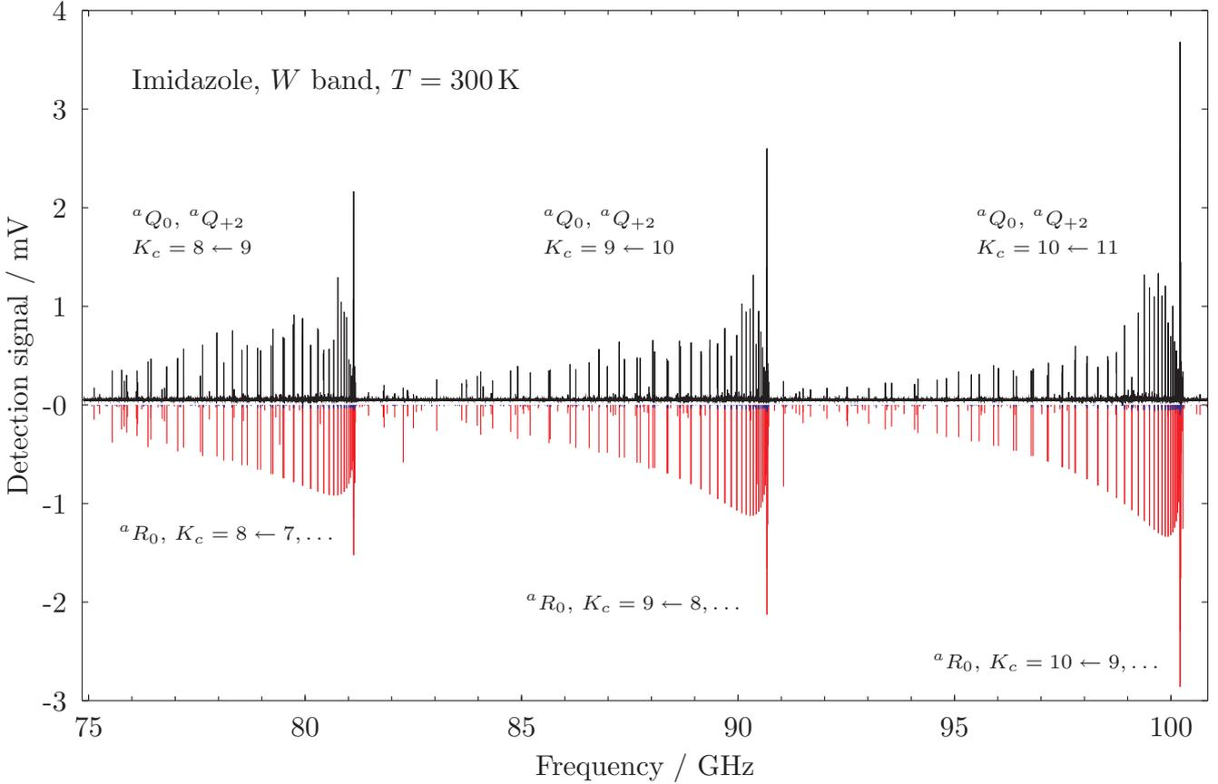
**Fig. 3.** Recording (black trace) of the imidazole rotational spectrum in the 3 mm region taken with the *W*-band segmented chirped-pulse spectrometer at DESY. The red histogram (inverted) indicates the predicted positions of the *a*-type lines computed using the spectroscopic parameters of Table 2. The *b*-type transitions (blue trace) are very weak and barely visible in the used *y*-axis scale.
