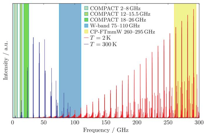
**Fig. 1.** Frequency intervals (shaded regions) covered by the measurements performed at DESY (COMPACT and W band) and at the University of Virginia (CP-FTmmW). Two calculations of the rotational spectrum of imidazole at 2 K (blue sticks) and 300 K (red sticks) are shown overlapped to highlight the spectral sampling.
