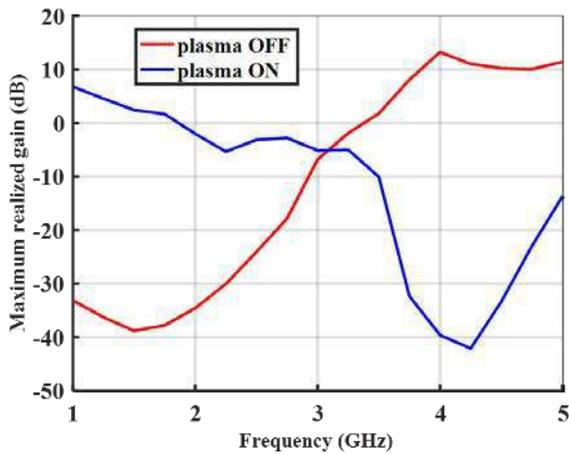
Fig. 8. Gain of the antenna in plasma OFF and ON cases.
