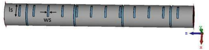
Fig. 5. Geometry of the slotted waveguide, small slots ( $l_s = 40 \text{ mm}$ ,  $w_s = 5 \text{ mm}$ ) for 4 GHz antenna and big slots ( $l_s = 150 \text{ mm}$ ,  $w_s = 5 \text{ mm}$ ) for 1 GHz antenna.
