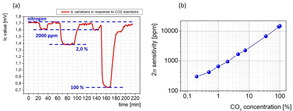
**Fig. 3:** prototype carbon dioxide calibration: (a) converted signal output variations following carbon dioxide injections. (b) calculated sensitivity as a function of the CO<sub>2</sub> concentration.
