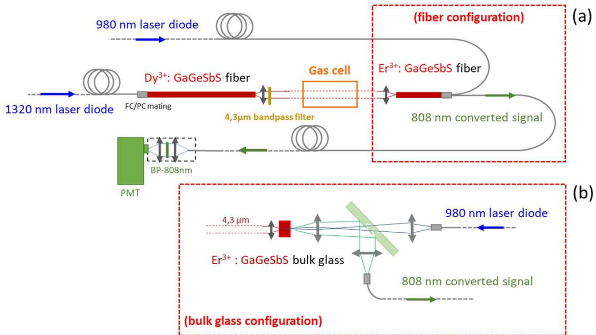
**Fig. 2:** Sensor scheme (a): fiber configuration; (b): bulk glass configuration
