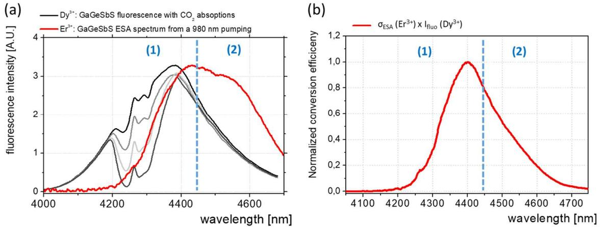
**Fig. 5:** (a):  $\text{Dy}^{3+}$ : GaGeSbS (with  $\text{CO}_2$  absorption dips for different  $\text{CO}_2$  concentrations) emission band and  $\text{Er}^{3+}$ : GaGeSbS excited state absorption spectrum. (b): spectral overlap between the  $\text{Er}^{3+}$  ESA and  $\text{Dy}^{3+}$  luminescence, indicating the wavelength conversion relative efficiency over this spectral domain.
