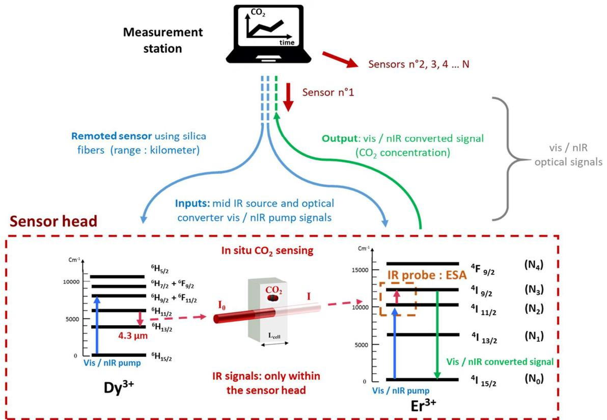
**Fig. 1:** overview of the MWIR CO<sub>2</sub> remote sensor based on rare earth luminescence as MWIR source (Dy<sup>3+</sup>) and as MWIR to visible wavelength converter (Er<sup>3+</sup>).
