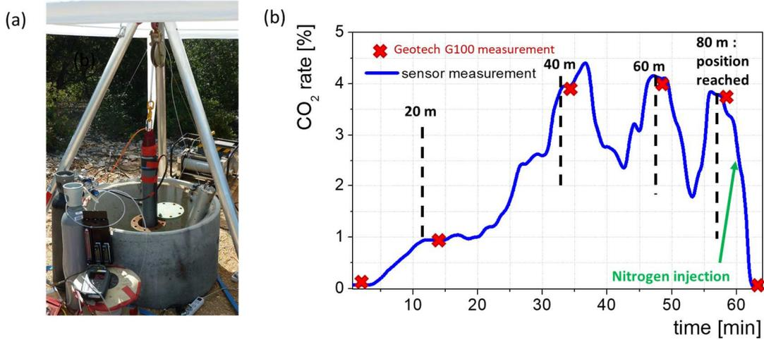
**Fig. 4:** (a): prototype (grey tube) being inserted in the pit; (b): CO<sub>2</sub> measurement performed with the all-optical sensor. Red crosses are the Geotech measurements points.
