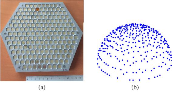
Fig. 2: (a) Picture of the reflectarray of maximum dimension  $8.8\lambda$  at 12 GHz. (b) Far field sampling points (total number of 353) selected by the DEIM and distributed on the measurement surface  $S$  (half a sphere).
