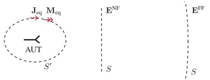
Fig. 1: Illustration of the antenna characterization problem. Equivalent electric and/or magnetic currents ( $\mathbf{J}_{\text{eq}}$  and/or  $\mathbf{M}_{\text{eq}}$ ) are placed on a surface  $S'$  enclosing the antenna under test (AUT). The near or far field ( $\mathbf{E}^{\text{NF}}$  or  $\mathbf{E}^{\text{FF}}$ ) is measured on a surface  $S$ .
