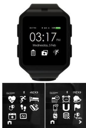
Figure A1. CareUp ® smartwatch home screen and watch panels for starting the BP measure and the calibration. In addition, the instruction manual to guide the user in the calibration and measurement procedure.
