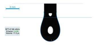
**Fig. 5** Sample image of measuring the surface tension of pure ethylene glycol with pendant drop method on Drop Shape Analyzer (KRUSS GmbH, Hamburg, Germany). Reused with permission from Ref. [32]
