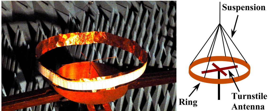
FIG. 10. Left: picture of the experimental set-up showing the turnstile antenna at the center of the rotating ring. The whole experiment takes place in an anechoic chamber. The radius of the ring is 15 cm. Right: principle of the experiment in order to exemplify the picture.
