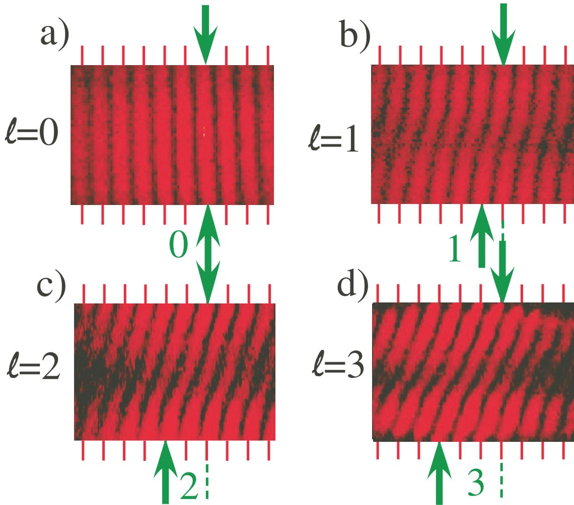
FIG. 7. Young's double slit interference: twisted interference patterns for beams with a)  $l = 0$  (usual double slit interference pattern); b)  $l = 1$ ; c)  $l = 2$ ; d)  $l = 3$ , for a vertical double slit orientation. The twist corresponds to  $l$  bright fringes of the interference pattern. The green arrows indicate the fringe order shift. From the twist, one can unambiguously determine the topological charge.
