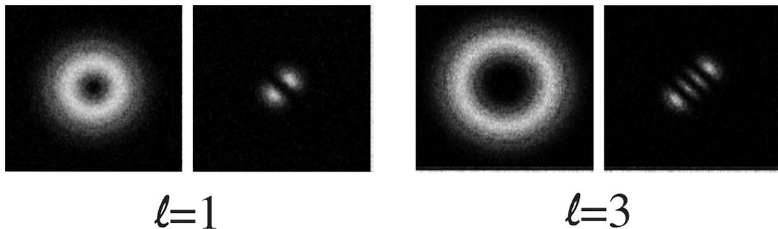
FIG. 2. Experimental transformation of a Laguerre Gaussian beam (left part) with  $\ell = 1$  and  $\ell = 3$  in a Hermite Gaussian beam (right part) using a single spherical lens. This spherical lens is tilted by  $20^\circ$  around the vertical axis. The number of zero of intensity of the Hermite Gaussian beam is equal to 1 and 3, corresponding to  $\ell = 1$  and  $\ell = 3$  respectively. This enables to clearly identify the topological charge of the Laguerre Gaussian beam.
