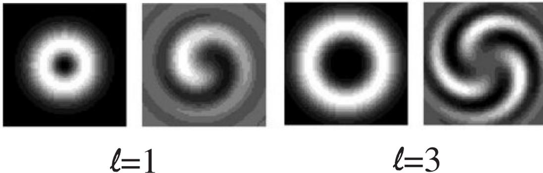
FIG. 4. Experimental interference (right) of a Laguerre Gaussian beam (left) with a plane wave for  $\ell = 1$  and  $\ell = 3$  Laguerre Gaussain beams respectively, showing the spiraling structure. The Laguerre Gaussian beams are here slightly diverging.
