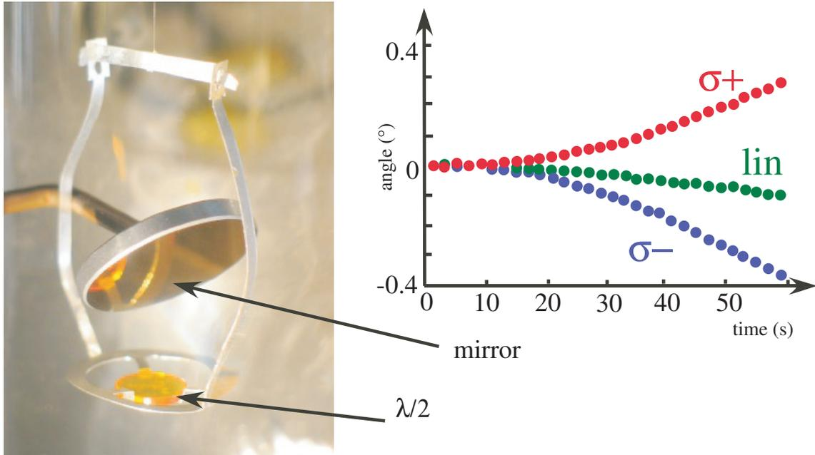
FIG. 9. Left: picture of the experimental set-up used to evidence the transfer of SAM to a halfwave plate. Right: uniform acceleration of the plate for a 10 Watts circularly right, circularly left and linearly polarized  $\text{CO}_2$  laser.
