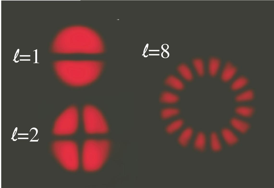
FIG. 5. Examples of interference patterns at the output of a Michelson interferometer. They indeed correspond to the interference between opposite topological charges ( $\ell = +1$  and  $\ell = -1$ ,  $\ell = +2$  and  $\ell = -2$ ,  $\ell = +8$  and  $\ell = -8$ ). It exemplifies the daisy flower like interference pattern.
