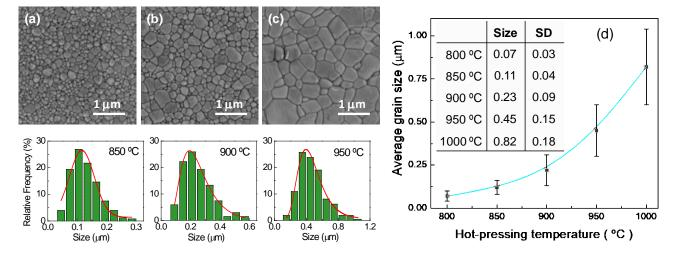
**Figure 2.** Scanning electron microscopy micrographs of ceramics of composition 1 ( $Bi_{0.62}Pb_{0.38}Fe_{0.52}Mn_{0.1}Ti_{0.38}O_3$ ) obtained by hot-pressing at (a) 850 °C, (b) 900 °C and (c) 950 °C, along with the resulting size distributions in each case. (d) Evolution of the average grain size with the sintering temperature (standard deviations, SD, are given as error bars). Grain sizes (µm) are given in the inserted table.
