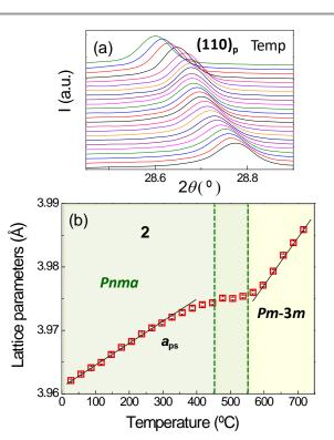
**Figure 6.** Temperature evolution of XRD profiles using  $CuK_{\beta}$  around the (110)<sub>p</sub> reflection (pseudocubic index) for powder sample of composition 2 (Bi<sub>0.62</sub>Pb<sub>0.38</sub>Fe<sub>0.47</sub>Mn<sub>0.15</sub>Ti<sub>0.38</sub>O<sub>3</sub>) after slow cooling. (b) Temperature evolution of the lattice parameter obtained from Le Bail analysis assuming to be pseudo-cubic ( $a_{ps}$ ). Colored regions indicate different polymorphs.
