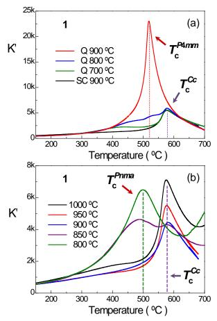
**Figure 9.** Temperature dependences of the relative permittivity (K') at 1 MHz during heating for ceramics of composition 1 ( $Bi_{0.62}Pb_{0.38}Fe_{0.52}Mn_{0.1}Ti_{0.38}O_3$ ). (a) Samples after thermal treatment at 900 °C with slow cooling (SC 900 °C) or quenching from increasing temperatures (Q700 °C, 800 °C, 900 °C). (b) Samples obtained at different hot-pressing temperatures (dashed lines and  $T_C$  are Curie temperatures).
