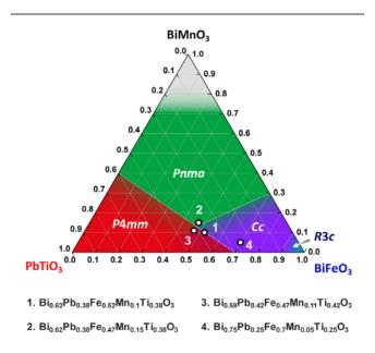
**Figure 1.** Schematic phase diagram of the BiFeO<sub>3</sub>-BiMnO<sub>3</sub>-PbTiO<sub>3</sub> ternary system, where MPB regions are highlighted and nominal compositions under study indicated with closed circles.
