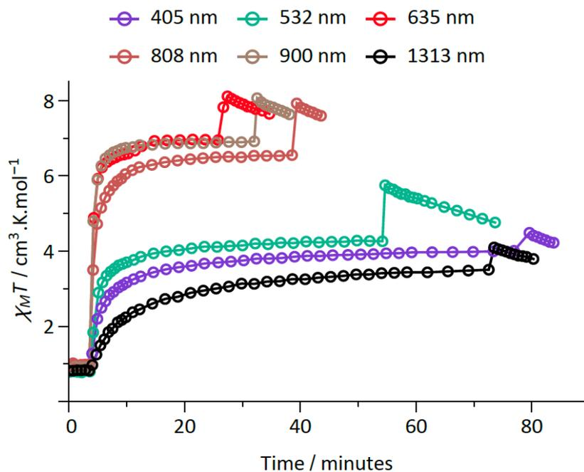
**Fig. 3.** Measurement of the  $\chi_M T$  product *versus* time under laser light irradiation (ca. 5 mW/cm<sup>2</sup>) at 20 K for the compound **2**. The first jump corresponds to the moment the light is switched on (photomagnetic effect) while the second jump corresponds to the moment the light is switched off and the temperature of the sample decreases.
