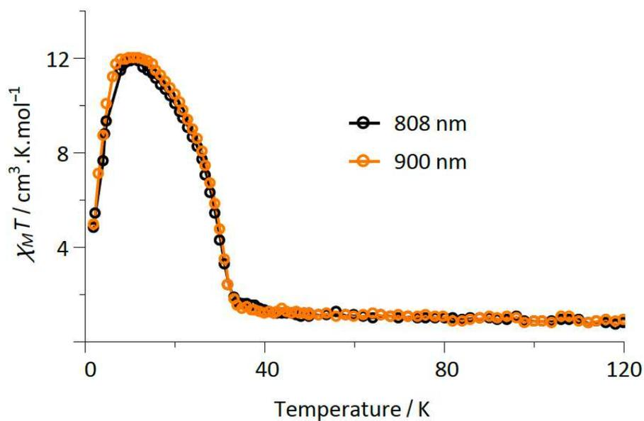
**Fig. 4.** Measurement of the  $\chi_M T$  product after laser light irradiation at 20 K ( $H = 1T$ ). The sample is measured from 2 to 100 K at 0.4 K/min.
