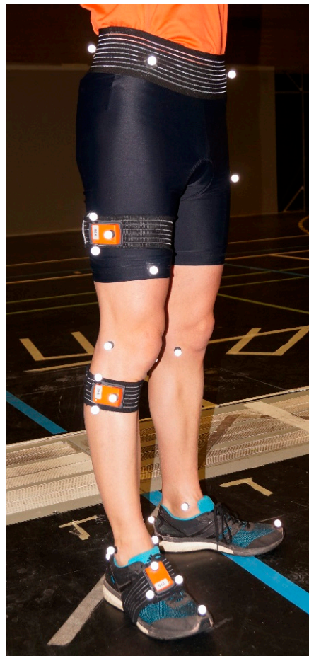
Figure 1. Subject equipped with an inertial measurement unit (IMU) and reflective markers.
