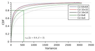
**Figure 4** CDFs of the Merged population depending of CU size for the sixth frame of the sequence *BasketballDrive*. Under a specific probability  $\Delta$ , a variance threshold can be extracted from the inverse CDF curve to classify a block as Merged.
