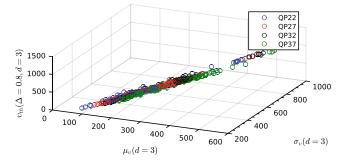
**Figure 5** Variance thresholds  $v_{th}(d = 3, \Delta = 0.8)$  versus the mean  $\mu_{v}(d = 3)$  and the standard deviation  $\sigma_{V}(d = 3)$  of CUs 8 × 8 variances. For a fixed value of  $\Delta$ , the variance threshold values form a plane (independently of the QP value).
