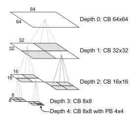
**Figure 1** Quad-tree structure of a Coding Tree Unit (CTU), divided into Coding Units (CUs) and Prediction Units (PUs) (dimensions in luminance pixels).
