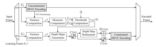
**Figure 9** Diagram of the Probabilistic proposed energy reduction scheme. The Learning Frames ( $F_L$ ) are encoded with a full RDO process (unconstrained) and the block variances of the resulting quad-tree decomposition are used to compute the set of thresholds  $v_{th}(d)$ . The
