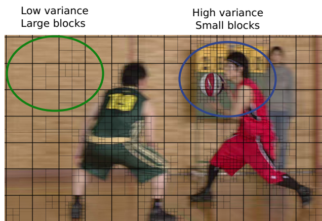
Figure 3 Quad-tree partitioning of the 6th HEVC intra coded frame of the BasketballDrive sequence. The green (resp. blue) circle shows that the lowest (resp. highest) variance regions tend to be encoded with larger (resp. smaller) units.
