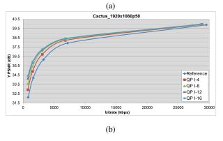
Fig. 1. R-D curves of non-Intra frames according to Intra QP offsets with (a) *Kimono* and (b) *Cactus* sequences
