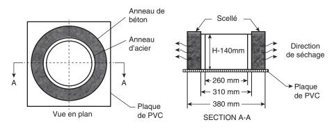
FIGURE 3. Geometry of the steel and concrete rings used in this study (18).
