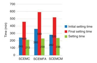
FIGURE 5. The initial times of setting, the final of setting and the setting time of SCEMs studied.
