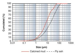
FIGURE 1. Laser granulometry of calcined mud and Fly ash.
