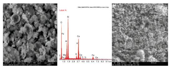
FIGURE 2. SEM and EDS analysis of calcined mud.
