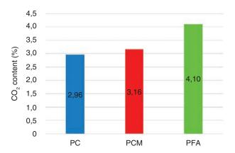
Figure 11.  $CO_2$  content of the mortar pastes studied.
