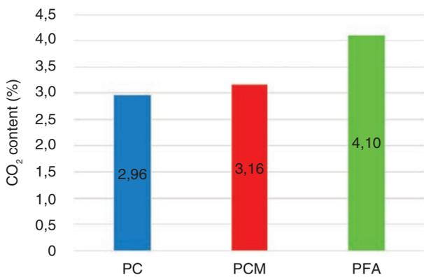
FIGURE 11. CO<sub>2</sub> content of the mortar pastes studied.
