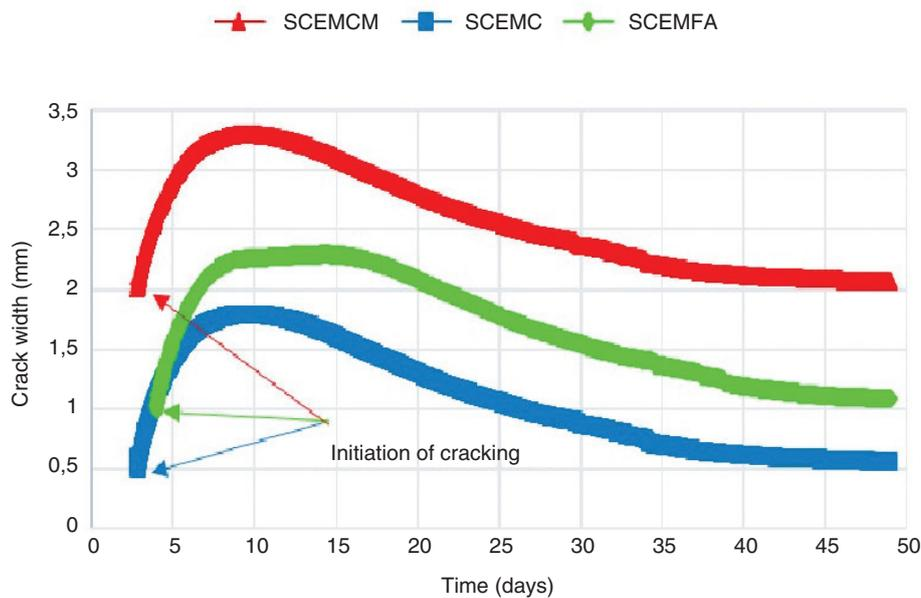
FIGURE 16. Measuring crack widths using a crack sensor.
