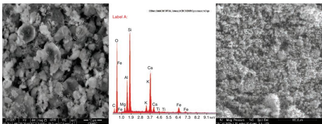
FIGURE 2. SEM and EDS analysis of calcined mud.
