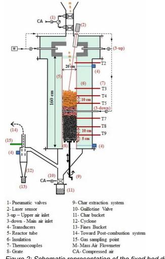
802 Figure 2: Schematic representation of the fixed bed downdraft reactor
