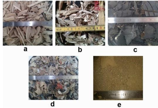
**Qe**798Figure 1: Photos of the fuels - scale unit in cm. a) Poplar wood chips, b) SRF wood chips, c) SRF Tire799chunks, d) SRF Plastic fluff, e) SRF Sewage sludge powder.
