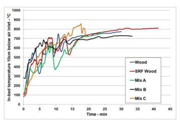
Figure 3: In-bed temperature measurement located 10cm below air inlet during gasification test for each fuel
