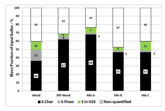
817 Figure 7: Mass balance of sulfur after gasification for each fuel
