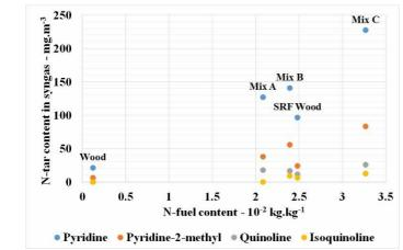
813• Pyridine • Pyridine-2-methyl • Quinoline • Isoquinoline814Figure 6: N-tar concentration in the producer gas versus N-fuel concentrations in the fuels
