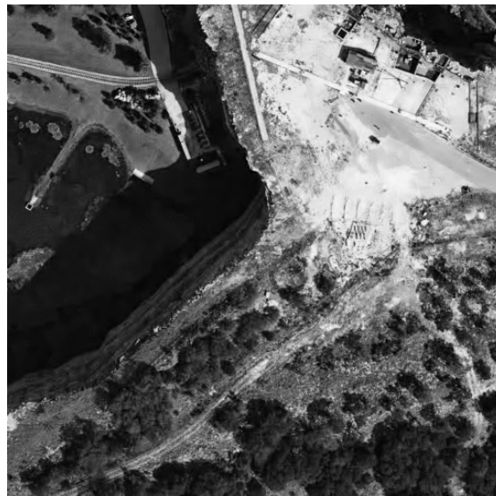
Figure 8. Filtered noisy image by 3D-DCT ( \beta = 3.0 ) with reference transformed by the first order polynomial ( \text{PSNR}_{\text{out}} = 34.73 dB; \text{PHVSM}_{\text{out}} = 38.05 dB).
