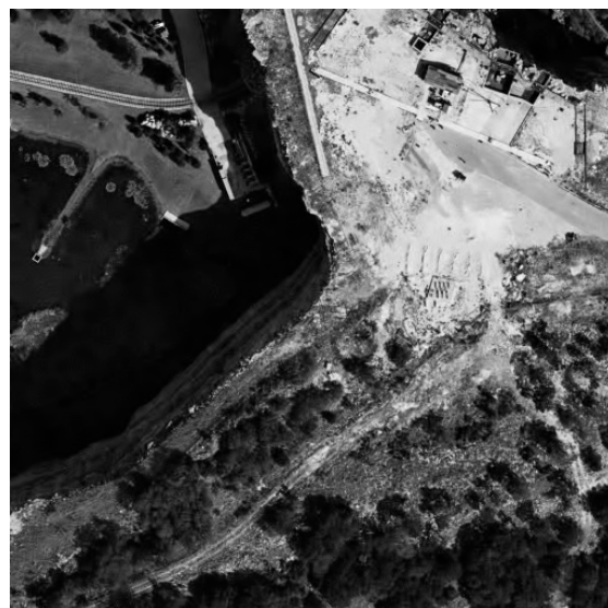
Figure 9. Filtered noisy image by 3D-DCT ( \beta = 3.0 ) with reference transformed by second order polynomial ( \text{PSNR}_{\text{out}} = 35.34 dB; \text{PHVSM}_{\text{out}} = 39.24 dB).
