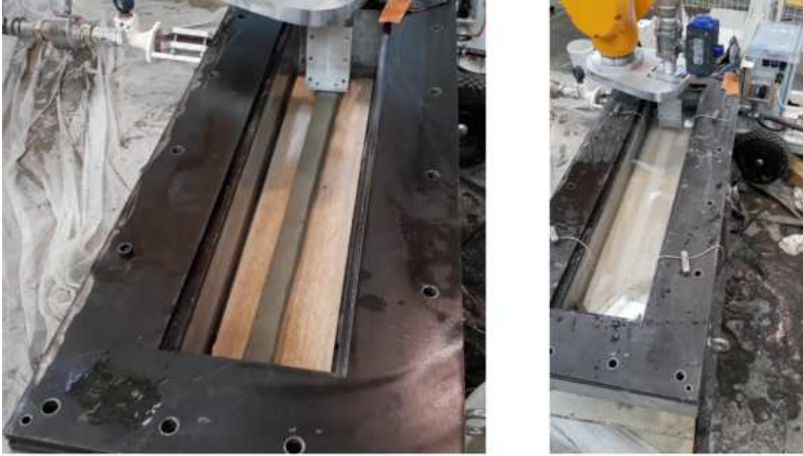
190 Fig. 2: Ongoing 3D printing of mortar –left: sample printed in air, right: sample printed in water.
