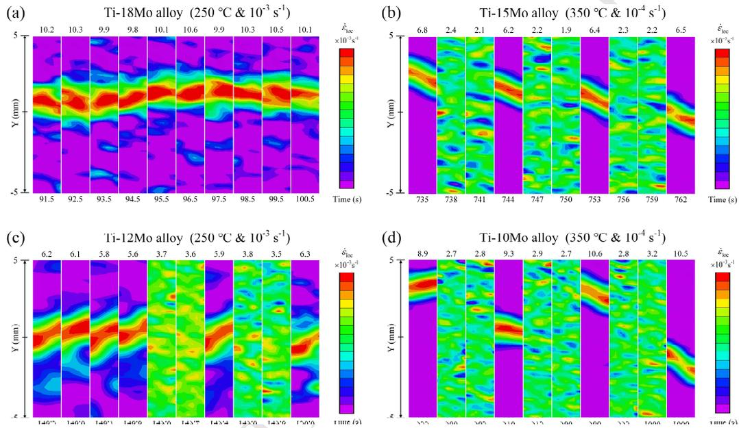
**Fig. 4.** Several typical propagation characteristics of PLC bands.
