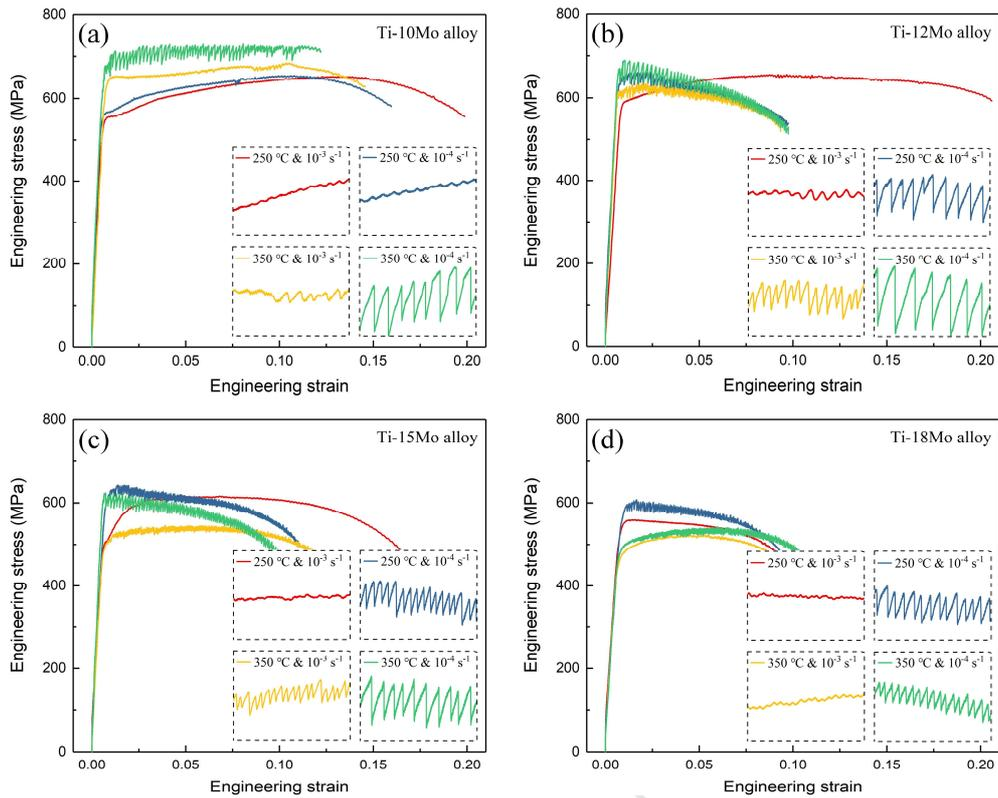
**Fig. 3.** Engineering stress-strain curves of Ti- $x$ Mo alloys at the temperature range of 250-350 °C with strain rates from the order of  $10^{-3} \text{ s}^{-1}$  to  $10^{-4} \text{ s}^{-1}$ .
