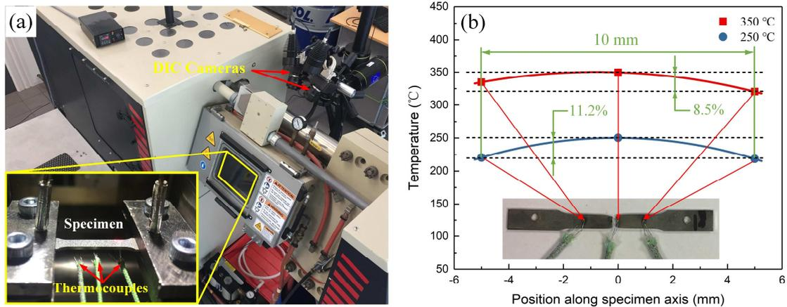
**Fig. 2.** Gleeble 3500 testing machine coupled with DIC for Ti-xMo alloys tensile tests at elevated temperatures (a) and temperature distribution along specimen axis (b).
