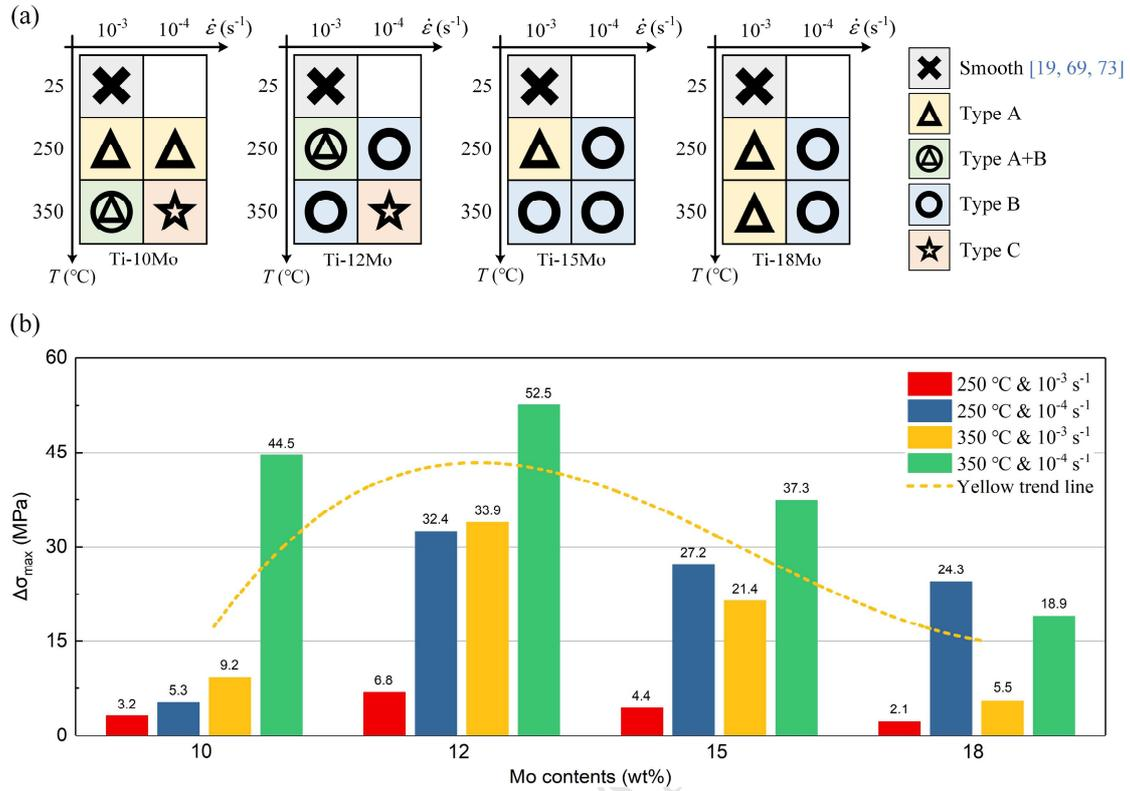
**Fig. 7.** Summary of serration types (a) and maximum stress drop magnitude  $\Delta\sigma_{max}$  (b) in the
