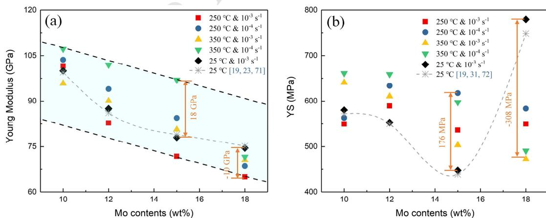
**Fig. 6.** Young modulus (a) and 0.2% offset yield strength (YS) (b) of Ti-xMo alloys at the temperature
