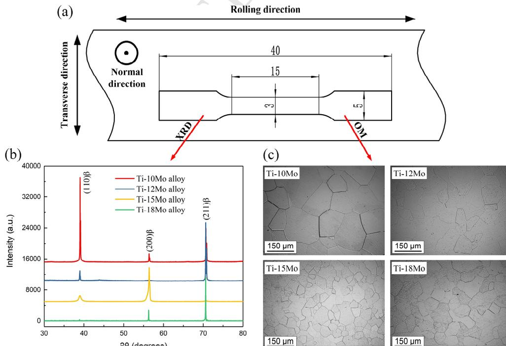
**Fig. 1.** Sample size (a), XRD (b) and OM (c) observations of Ti-xMo alloys.
