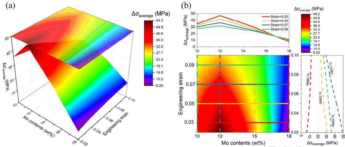
**Fig. 8.** 3D surface plot with projection map (a) and the contour plot with some fundamental evolution characteristics of average stress drop magnitude (b) at various Mo contents and engineering strains under the experimental condition ( $350\text{ }^{\circ}\text{C}$  &  $10^{-4}\text{ s}^{-1}$ ).
