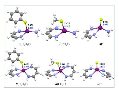
**Figure 8**. Optimised geometries of the  $A(C_6H_5F)$ ,  $A(CH_3F)$ ,  $AF^-$ ,  $B(C_6H_5F)$ ,  $B(CH_3F)$  and  $BF^-$  models. Interatomic distances are given in Å; in black, with D3 corrections; in blue, without D3 corrections.
