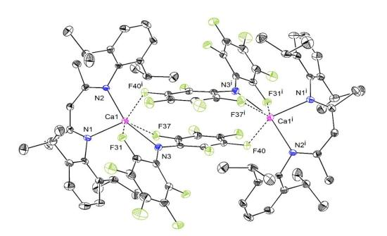
**Figure 6.** ORTEP representation of the molecular solid-state structure of  $[\{BDI^{DiPP}\}CaN(C_6F_5)_2]_2$  (72). Ellipsoids at the 50% probability level. H atoms and non-interacting benzene molecule omitted for clarity. Ca···F interactions depicted in dashed bonds. Selected bond lengths (Å): Ca1-N1 = 2.3066(19), Ca1-N2 = 2.3465(18), Ca1-N3 = 2.3880(19), Ca1-F40<sup>i</sup> = 2.5325(15), Ca1-F31 = 2.5559(15), Ca1-F37 = 2.7120(17).
