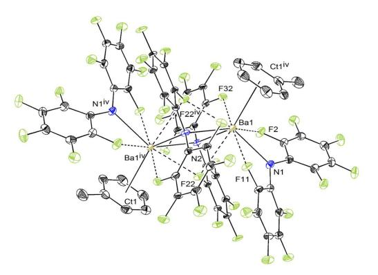
**Figure 5.** ORTEP representation of the molecular solid-state structure of  $[Ba\{\mu-N(C_6F_5)_2\}\{N(C_6F_5)_2\}\{N(C_6F_5)_2\}\}$ . toluene]<sub>2</sub> (62). Ellipsoids at the 50% probability level. H atoms omitted for clarity. Ba···F interactions depicted in dashed bonds. Selected bond lengths (Å): Ba1-N1 = 2.740(3), Ba1-F11 = 2.825(2), Ba1-F32 = 2.832(2), Ba1-N2 = 2.871(4), Ba1-F2 = 2.910(3), Ba1-F22<sup>iv</sup> = 2.923(3), Ba1-N2<sup>iv</sup> = 2.951(3), Ba-F22 = 3.014(3).
