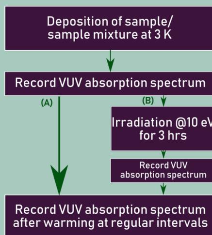
**Figure 2.** Flow chart showing the experimental procedure for the two sets of photoabsorption studies: (A) Benzonitrile and (B)  $\text{NH}_3$ - $\text{O}_2$  ices- Hydroxylamine
