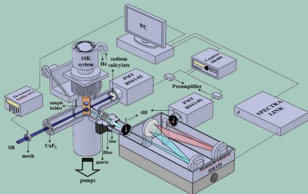
**Figure 1.** Station design at the BL03A1 beamline (Taken from the NSRRC webpage <http://efd.nsrcc.org.tw/EFD.php?num=238>)
