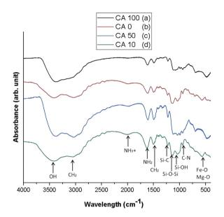
**Fig. 8.** FTIR spectra of the different solid residues obtained during the synthesis of the different composite materials (a) CA100, (b) CA0, (c) CA50, and (d) CA10.
