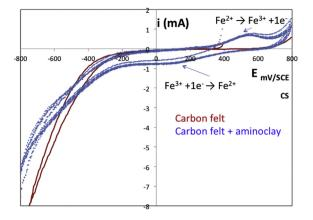
**Fig. 9.** Current–potential plot of the composite material in 0.05 M Na<sub>2</sub>SO<sub>4</sub> supporting electrolyte, at pH = 3 under inert atmosphere (N<sub>2</sub>) and 30 °C, obtained with graphite felt (continuous line) or CA100 composite (dashed line) as working electrode, Pt counter electrode, and saturated calomel electrode with a scan rate of 10 mV s<sup>-1</sup>. SCE, saturated calomel electrode.
