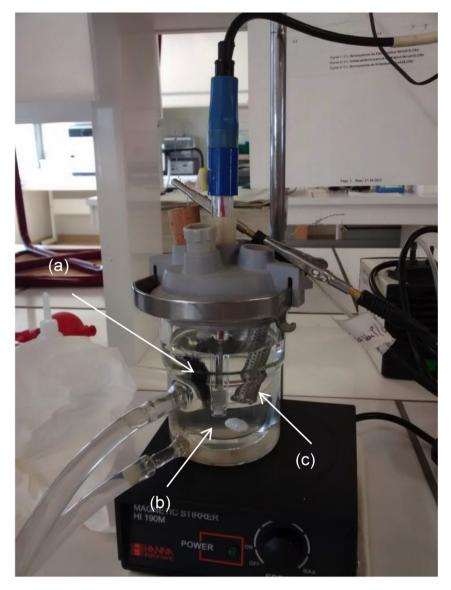
Fig. 2. Experimental setup used for the current-potential curves and the electrolysis tests: (a) cathode (composite material or carbon felt alone), (b) reference electrode (saturated calomel electrode), and (c) counter electrode (Pt).
