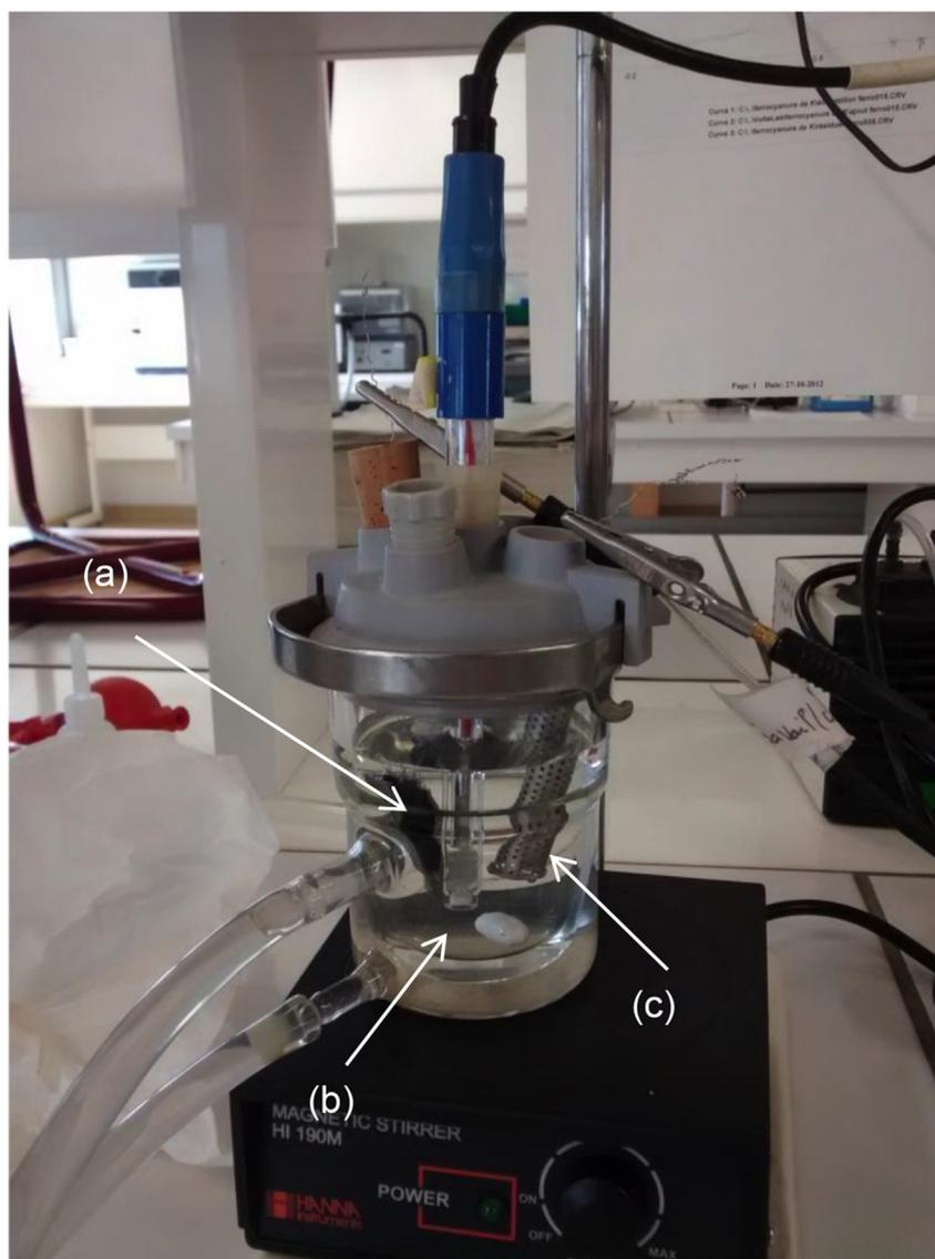
**Fig. 2.** Experimental setup used for the current–potential curves and the electrolysis tests: (a) cathode (composite material or carbon felt alone), (b) reference electrode (saturated calomel electrode), and (c) counter electrode (Pt).
