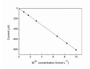
**Fig. 2.** Current *versus* Bi(III) concentration obtained by linear sweep voltammetry on rotating disk electrode (glassy carbon) in solutions of Bis-Tris at pH 13 at 1500 rpm and 5 mV s<sup>-1</sup>.
