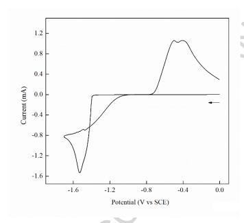
**Fig. 3.** Cyclic voltammogram obtained at a glassy carbon electrode ( $S=7 \text{ mm}^2$ ) of a solution of Bi<sub>2</sub>O<sub>3</sub> solubilized at 1 mol L<sup>-1</sup> by 1.1 equivalents of Bis-Tris at pH 14. Scan rate 100 mV s<sup>-1</sup>
