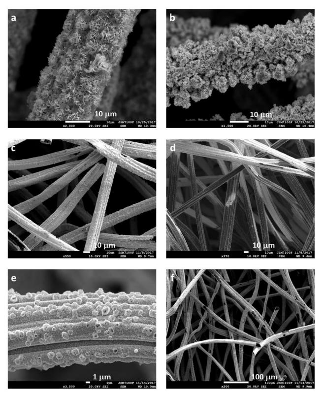
**Fig. 4.** SEM images of Bi modified graphite felt prepared according to experimental conditions given in Table 3. a) entry 4 (inside) b) entry 4 (external surface) c) and d) entry 6 (inside) e) f) entry 7 (inside).
