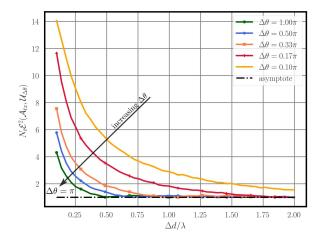
Fig. 6. Numerical evaluation of  $\mathcal{E}(A_{tx}, \mathcal{U}_{\Delta\theta})$  for increasing  $\Delta\theta$  with fixed number of antennas  $N_t=16$ . The lower, the better.
