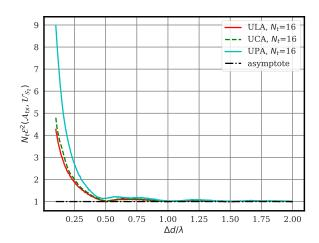
Fig. 2. Numerical evaluation of  $\mathcal{E}(A_{tx}, \mathcal{U}_{S_2})$  for various array types and increasing antenna spacing  $\Delta d$ . The values are normalized so the asymptote is 1
