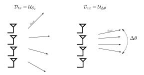
Fig. 4. On the leftmost side, uniform distribution of the rays on the unit sphere  $\mathcal{U}_{\mathcal{S}_2}$ . On the rightmost side, constrained distribution of the rays with solid angle  $\mathcal{U}_{\Delta\theta}$
