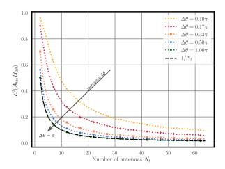
Fig. 5. Numerical evaluation of  $\mathcal{E}(A_{tx}, \mathcal{U}_{\Delta\theta})$  for increasing  $\Delta\theta$  with fixed half-wavelength antenna spacing. The lower, the better.
