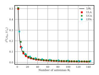
Fig. 3. Numerical evaluation of  $\mathcal{E}(A_{tx}, \mathcal{U}_{S_2})$  for various antenna arrays at the half wavelength. The lower, the better.
