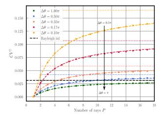
Fig. 7. Comparison between (7), simulated  $CV^2$  and correlated Rayleigh, the dashed, squared and dotted lines respectively. A  $16\times 2$  ULA setup is considered. Uniform distribution of DoDs and DoAs with constrained DoDs and complex Gaussian gains. The large-scale factor is normalized.
