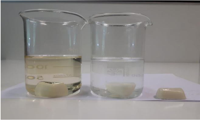
Figure 3. The three samples of G16O20 mixture preserved (from left to right) in sunflower oil, deionized water and air.
