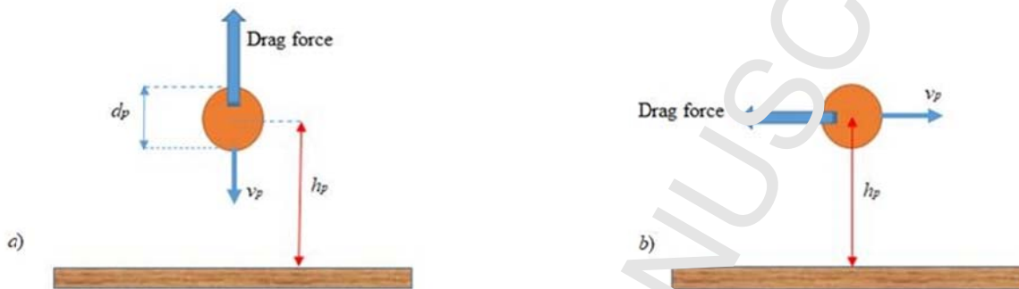
Figure 8. Drag coefficient when (a) particle moves toward wall, (b) particle moves parallel to wall.
