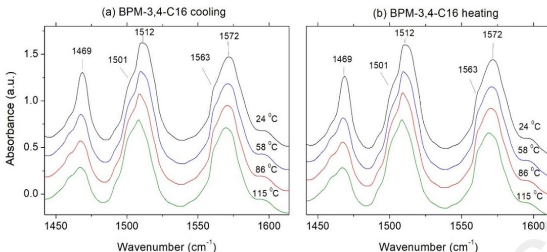
**Figure 11.** Temperature dependence of the IR absorption spectra of BPM-3,4-C16 thin films on cooling (a) and heating (b). Note that for clarity the spectra are separated along the absorbance axis.
