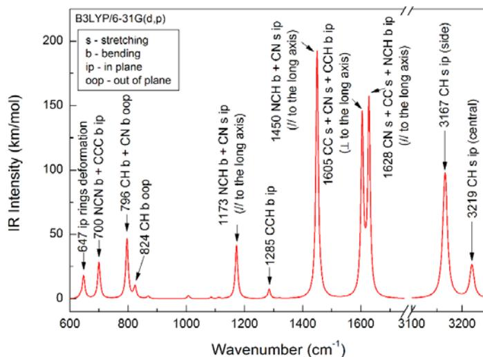
**Figure 3.** Calculated IR spectra of the molecular core.
