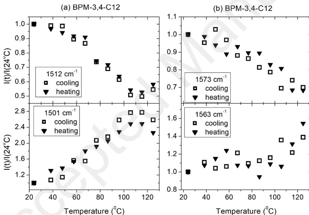
**Figure 14.** Temperature dependence of the integral intensity of the spectral features for thin layer of BPM-3,4-C12 on cooling and heating: (a) side-band at  $1501\text{ cm}^{-1}$  and main band at  $1512\text{ cm}^{-1}$  and (b) side-band at  $1563\text{ cm}^{-1}$  and main band at  $1573\text{ cm}^{-1}$ .
