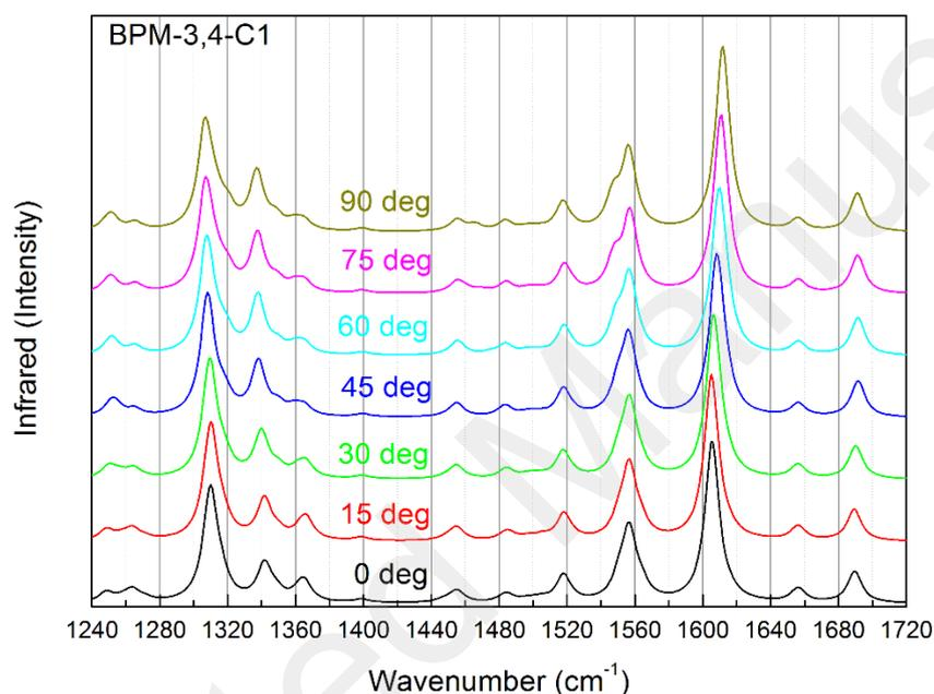
**Figure 6.** The simulated IR spectra of BPM-3,4-C1
