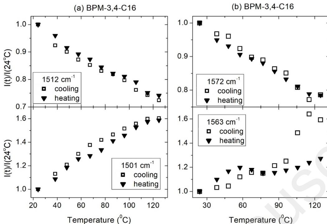
**Figure 12.** Temperature dependence of the integral intensities of spectral bands for thin layer of BPM-3,4-C16 on cooling and heating: (a) side-band at 1501  $\text{cm}^{-1}$  and main-band at 1512  $\text{cm}^{-1}$  and (b) side-band at 1563  $\text{cm}^{-1}$  and main-band at 1572  $\text{cm}^{-1}$ .
