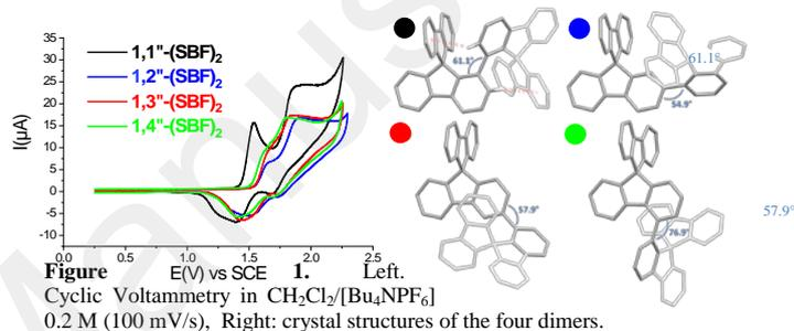
**Figure 1.** Cyclic Voltammograms (CV) of **1,2''-(SBF)<sub>2</sub>**, **1,3''-(SBF)<sub>2</sub>** and **1,4''-(SBF)<sub>2</sub>** in  $\text{CH}_2\text{Cl}_2$  [ $\text{Bu}_4\text{NPF}_6$ ] 0.2 M (100 mV/s), Right: crystal structures of the four dimers.
