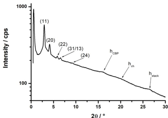
**Figure 7.** XRD pattern of **2b**, (C<sub>12</sub>dt)Pt(bpyCBP), recorded at 30 °C after cooling from the isotropic phase.
