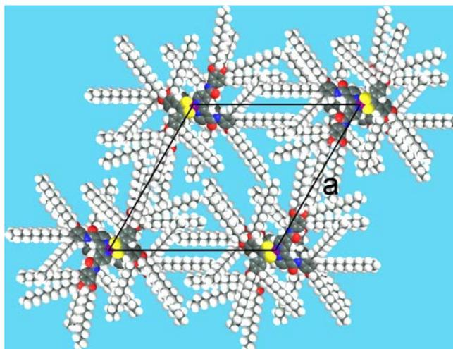
**Figure 6.** Proposed model for the organization of **2a** in the  $Col_h$  phase (Molecular diameter  $\sim 48$  Å (Dreiding model); atom: white = hydrogen, grey = carbon, blue = nitrogen, yellow = sulfur, purple = platinum, red = oxygen).
