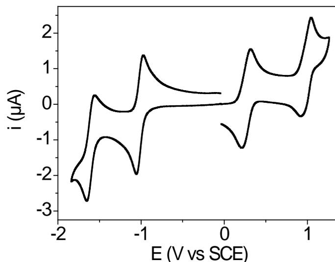
**Figure 3.** Cyclic voltammogram of (ddd)Pt(bpyCBP) **1b** ( $\sim 10^{-3}$  M) in  $\text{CH}_2\text{Cl}_2$  containing 0.2 M  $\text{NBu}_4\text{PF}_6$  at a 1-mm disk carbon electrode. Scan rate is  $0.1 \text{ V s}^{-1}$  and  $T = 293 \text{ K}$ .
