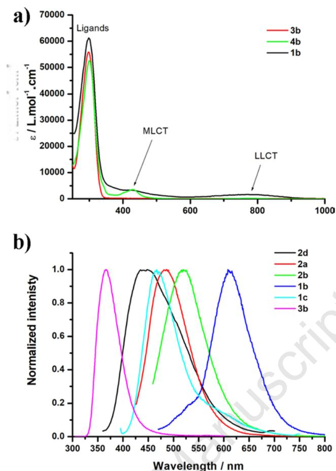
**Figure 2.** a) UV-Vis absorption spectra in  $\text{CH}_2\text{Cl}_2$  ( $C \sim 10^{-5} \text{ M}$ ) of **3b**, **4b** and **1b**; b) Normalized emission spectra in  $\text{CH}_2\text{Cl}_2$  ( $C \sim 10^{-5} \text{ M}$ ) of all the compounds upon excitation in the MLCT band (except for **3b**,  $\lambda_{\text{ex}} = 300 \text{ nm}$ ).
