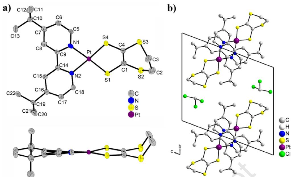
**Figure 1.** a) ORTEP diagram of **1c** from the top and from the side with 50% thermal contours for all atoms and the atomic numbering scheme. H atoms have been omitted for the sake of clarity; b) Projection of the crystalline structure along the *a* axis.
