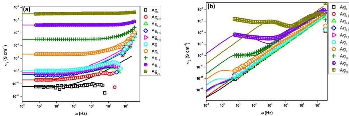
**Fig. 3 a)** The real part of conductivity  $\sigma_1$  and **b)** the imaginary part of conductivity  $\sigma_2$  as a function of the sample composition at 368 K. Open symbols represent the experimental data, the solid lines represents the RW model fitting.
