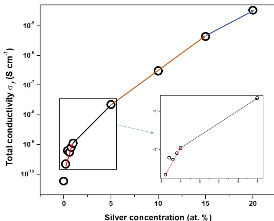
**Fig. 4** The total conductivity ( $\sigma_T$ ) as a function of Ag concentration at 368 K. Inset shows magnified image of the marked area. Open symbols represents the experimental value whereas solid line colored arrows represents the guideline for eyes.
