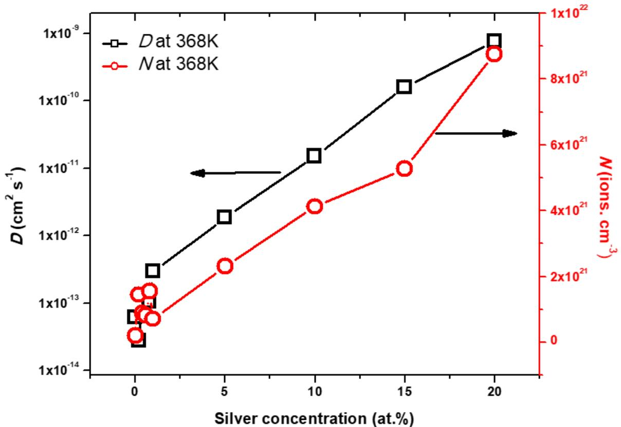
**Fig. 5** The diffusion coefficient ( $D$ ) and the mobile ion concentrations ( $N$ ) calculated using RW model plotted as a function of Ag concentration at 368 K. Open symbols represent the calculated values whereas solid line represent the guideline for eyes.
