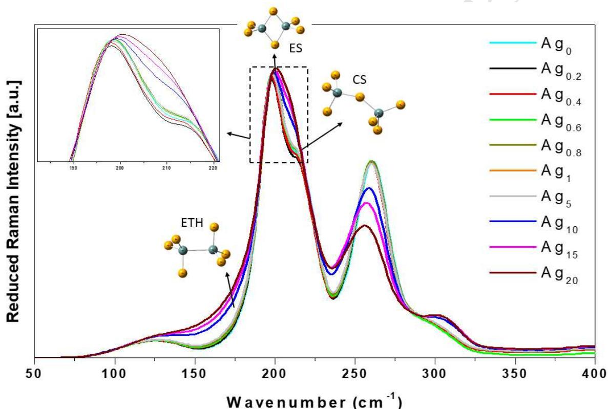
**Fig. 9** Reduced Raman spectra of  $Ag_x(Ge_{16}Sb_{12}Se_{72})_{100-x}$  (where  $x = 0$  to 20), inset the magnified image of dotted block. The orange colored balls and cyan colored balls in ball stick models are Se and Ge respectively.
