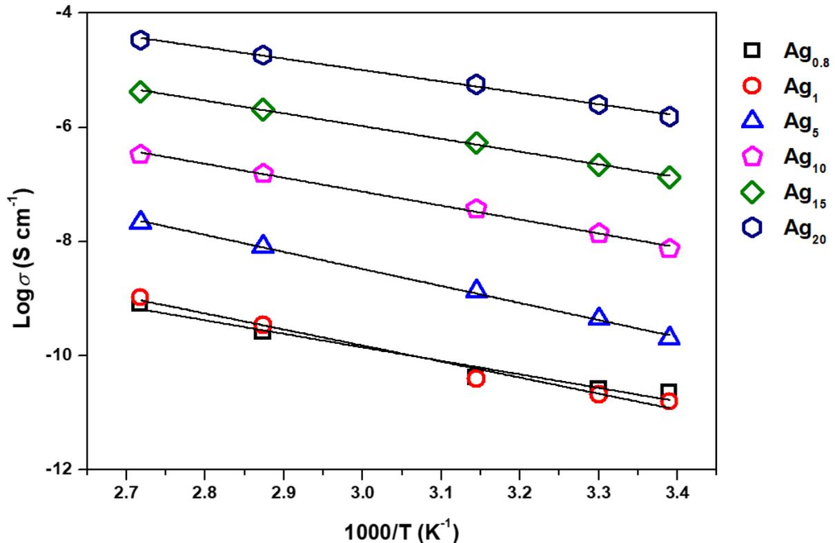
**Fig. 6** The temperature dependence of  $\sigma_T$ . The open circles represent the experimental  $\sigma_T$ . The solid line represents the fitting to Arrhenius Eq. (4).
