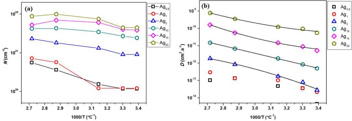
**Fig. 7 a)** The concentration of the mobile ions ( $N$ ) vs reciprocal of temperature, **b)** diffusion coefficient ( $D$ ) vs reciprocal of temperature, in both a) and b) the open symbol represents the respective figs. calculated from RW model fitting to experimental data and the solid line in a) is the guideline for eye whereas in fig. b) exponential fit to the eq. 5.
