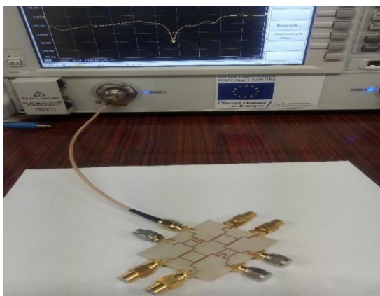
FIGURE 9. Photograph of the fabricated BM under test.
