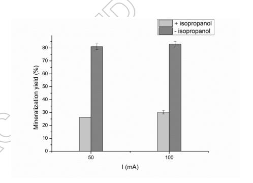
Figure 3 . Mineralization yield of AR18 as a function of the current intensity in presence (light grey bars) and absence (dark grey bars) of isopropanol (1M), with 40 mg.L $^{-1}$  Fe<sub>3</sub>O<sub>4</sub>, at pH 3, in 250 mL Na<sub>2</sub>SO<sub>4</sub> 0.05M
