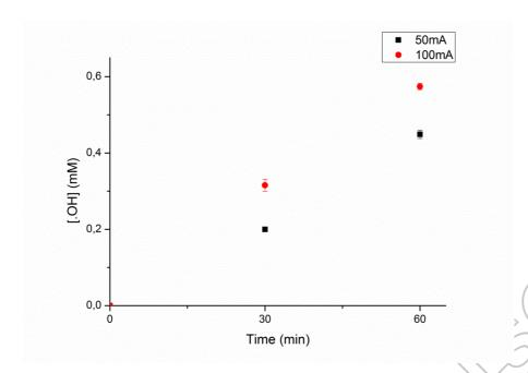
Figure 2. Concentration of generated •OH as a function of the current density during 180 min of electrolysis, with DMSO 0.25M, 40 mg.L $^{-1}$  Fe<sub>3</sub>O<sub>4</sub>, at pH 3, in 250 mL Na<sub>2</sub>SO<sub>4</sub> 0.05M
