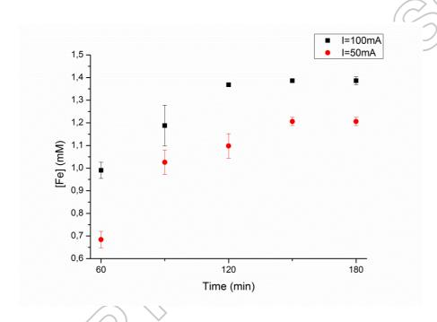
Figure 1. Investigation of Fe ion dissolution as a function of the current intensity during 180 min, with 40 mg.L $^{-1}$  Fe $_3$ O $_4$ , at pH 3, in 250 mL Na $_2$ SO $_4$  0.05M
