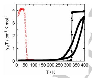
Figure 6. Thermal dependence of  $\chi_M T$  for 1 (full circles), 1.4MeNO<sub>2</sub> (full square). The thermal dependence of  $\chi_M T$  1.4MeNO<sub>2</sub> after light irradiation (660 nm, 5 mW) is represented with red squares.
