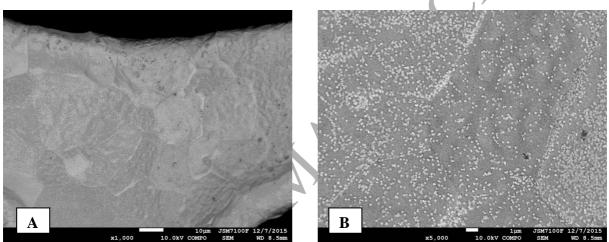
Figure 2: Scanning electron microscopy (SEM) images of Ag-nanoparticules on Ni foams (A  $\times$  1000, B  $\times$  5000) (Reproduced with modification from [49].)
