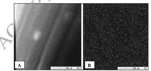
Figure 1: Scanning electron microscopy (SEM) images of palladium-loaded carbon felt: (A) the secondary electron image (SEI) of the felt surface and (B) the mapping of supported palladium from the energy-dispersive X-ray analysis (EDAX). (Reproduced with modification from [41].)
