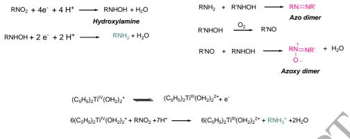
Scheme 2: Direct and catalytic reduction of nitro compounds
