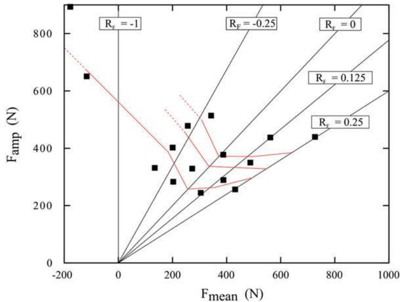
Fig. 8.3 Haigh diagram at 90 °C
