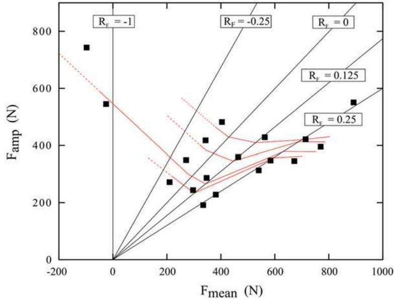
**Fig. 8.2** Haigh diagram at 23 °C
