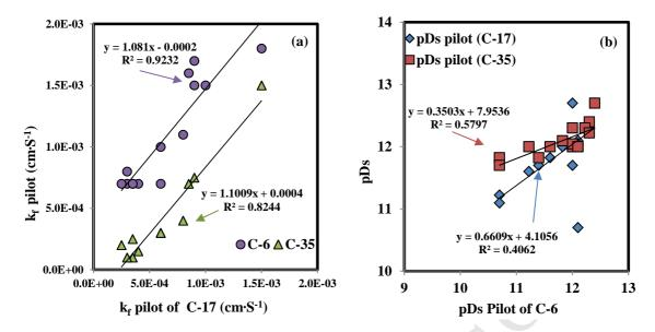
**Figure 6**: (a) Correlation among the fitted  $k_f$  values for full-scale pilot of virgin and aged GAC for the various compounds ( $k_f$  values have been discarded when the Biot number exceeded 100); (b) Correlation analysis of the  $pD_s$  values for full-scale pilot of aged GACs
