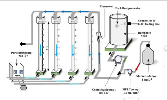
Figure 1: Schematic description of the full-scale pilot installation
