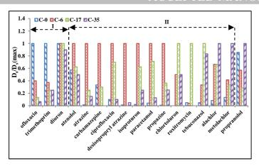
**Figure 3**: Relative surface diffusivities of micropollutants ( $D_s$  value compared to maximum  $D_s$  value of the four GACs) with various aged GACs (C-0, C-6, C-17 and C-35 represent respectively the virgin GAC and the aged GACs being in service for 6, 17 and 35 months). Two different groups of behaviors with exception of propranolol, labeled I to II, are identified.
