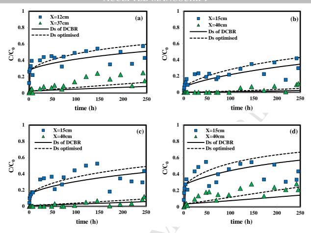
**Figure 5**: Breakthrough curves of atenolol with 4 GACs at the two depths: (a) C-0; (b) C-6; (c) C-17 and (d) C-35. Continued black line is HSDM modeling curve with  $D_s$  value obtained in DCBR setup, discontinued black line is HSDM modeling curve with optimized  $D_s$  value.
