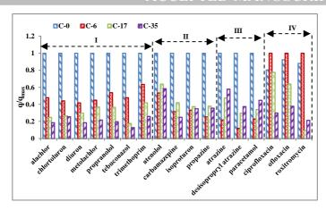
**Figure 2**: Relative adsorption capacities of micropollutants (q value compared to maximum q value of the four GACs) with various aged GACs (C-0, C-6, C-17 and C-35 represent respectively the virgin GAC and the aged GACs being in service for 6, 17 and 35 months). Four different groups of behaviors, labeled I to IV, are identified.
