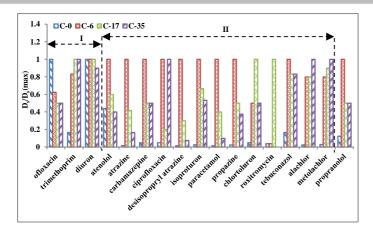
**Figure 7:** Time evolution of relative  $D_s$  values obtained from the fixed bed experiments. Group I and II are those defined in **Figure 3**.
