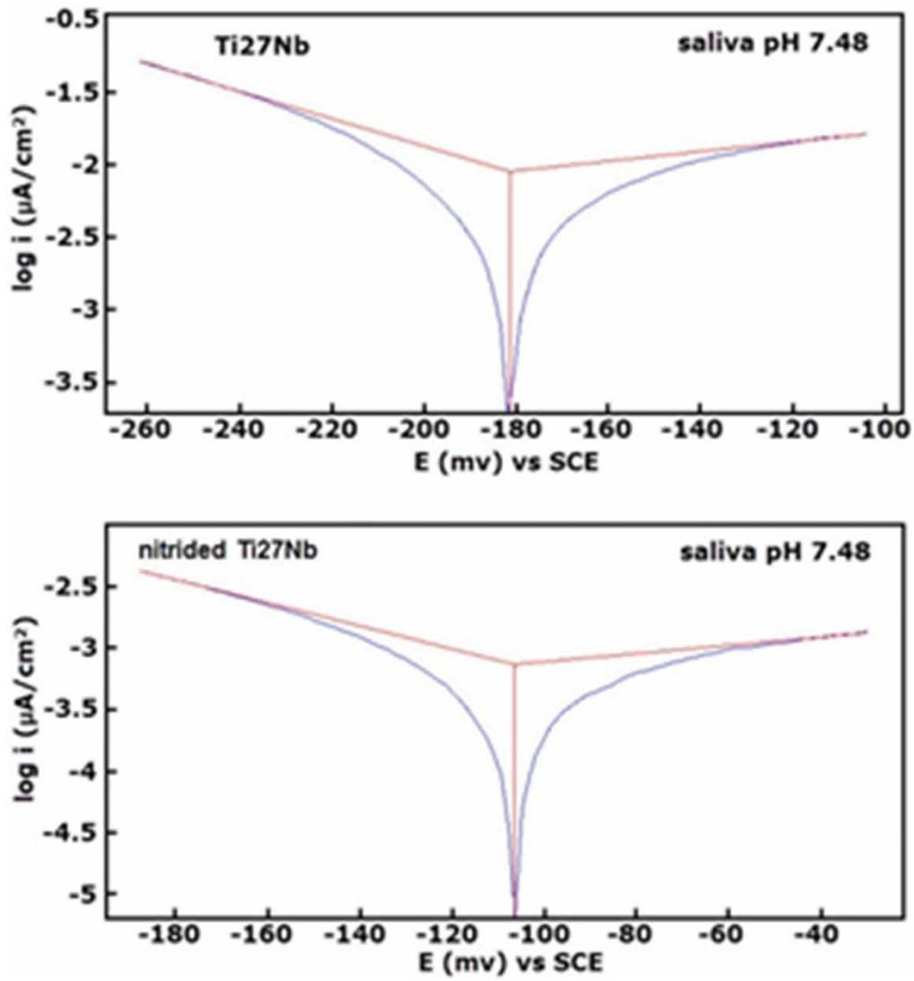
**Fig. 5** Tafel representations for the non-nitrified and nitrified Ti-27Nb alloy in Carter-Brugirard saliva at saliva pH = 7.48
