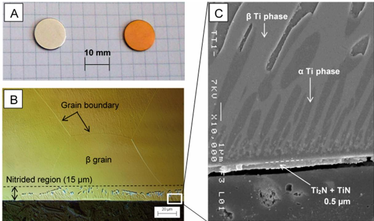
**Fig. 2 a** Photography of the samples: Ti-27Nb (grey colour) and nitrided Ti-27Nb (golden yellow colour). **b** Optical micrograph (polarized light) showing the cross-section microstructure. **c** SEM image showing the cross-section microstructure in surface of the nitrided Ti-27Nb alloy. The very thin uniform nitrided layer (0.5μm in thickness) is visible at the external zone
