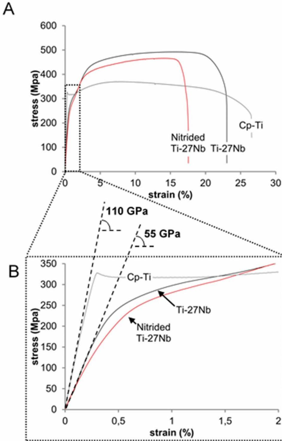
**Fig. 4 a** Stress strain tensile curves of Cp-Ti, nitrided and non-nitrided Ti-27Nb alloy. **b** The Young's modulus measured at the origin of the tensile curves
