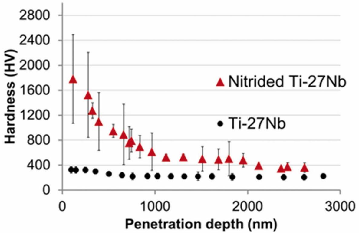
**Fig. 3** Hardness profiles of nitrided and non-nitrided Ti-27Nb alloy
